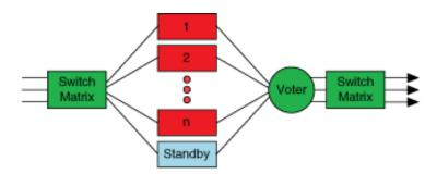
Other drawbacks of this approach are the added complexity of deciding when to switch and of a switch matrix that can reroute the signals correctly and efficiently.
