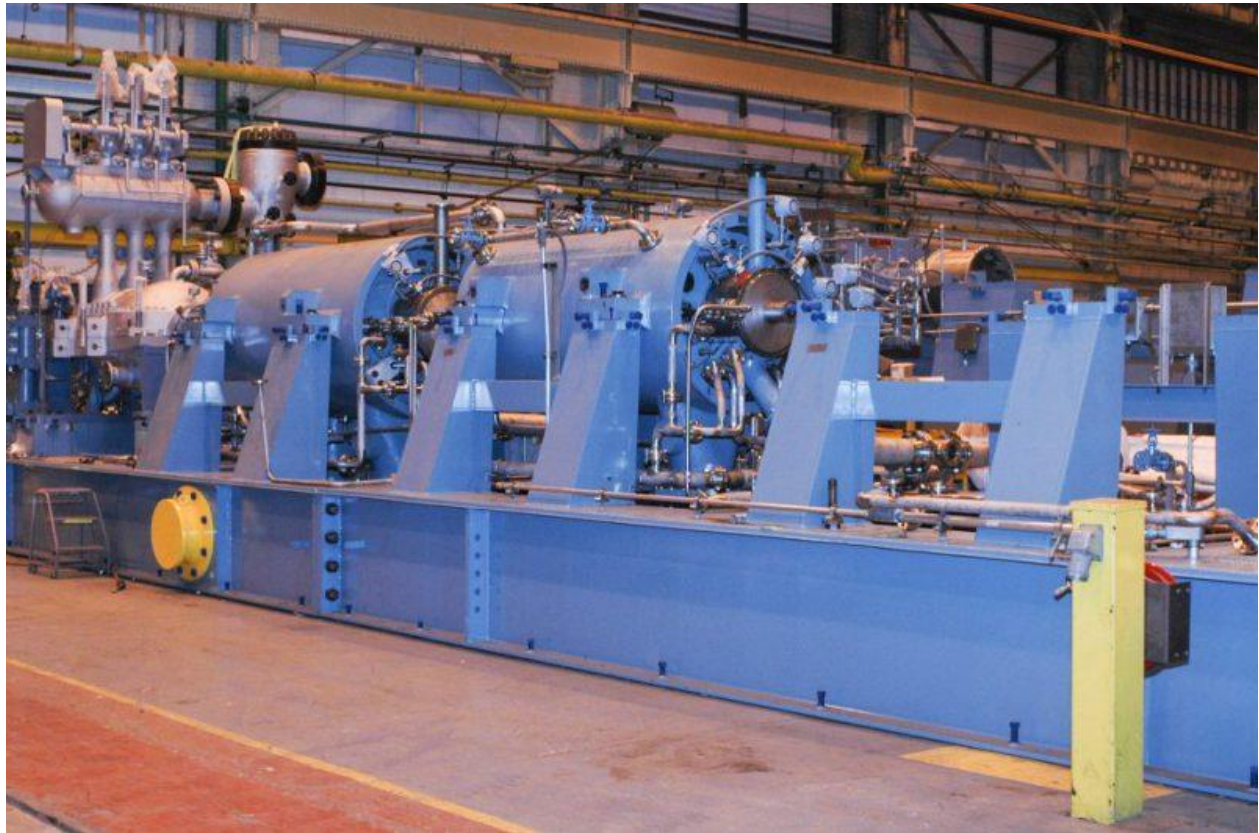
Steam Turbine Driven Gas Compression Train [Dresser Rand]
