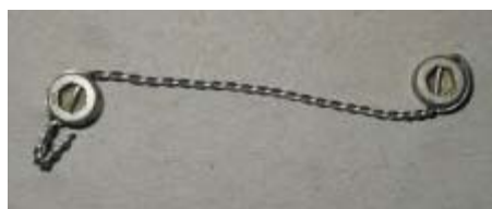
Figure 50: Example of the use of lock wire
