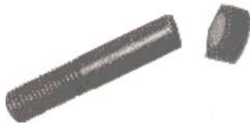
Figure 64: Brittle rupture of a screw
