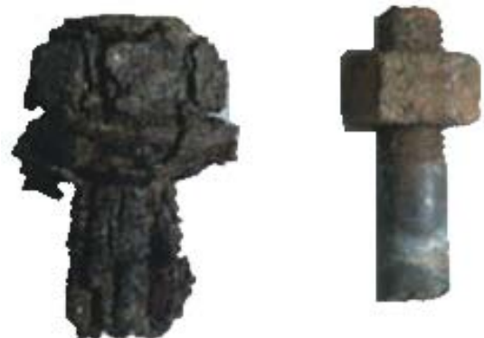
Figure 65: Example of corroded screws and nuts
