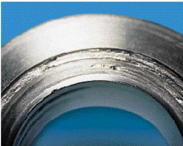
Figure 40: Surface condition of a part tightened using the cross method, with an impact wrench and an extension.
