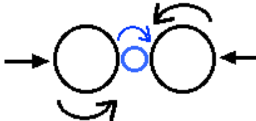
Figure 20: Roll bending of threads
