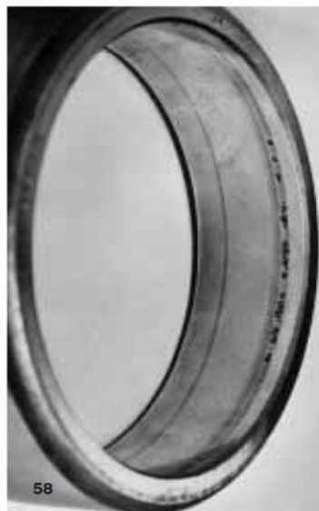
Fig 59 Flaked inner ring of a spherical roller bearing. The extent of the flaking around one entire raceway indicates that the axial load has been very heavy in relation to the radial load
